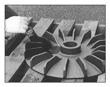
SYNTHETIC RUBBER BRUSH ON is a high performance liquid polyurethane that is used where application of product by brush is preferred. Once cured, it exhibits excellent resistance to impact, wear and chemicals providing considerable benefits when used in lining, repair and treatment applications. TYPICALLY USED ON:
