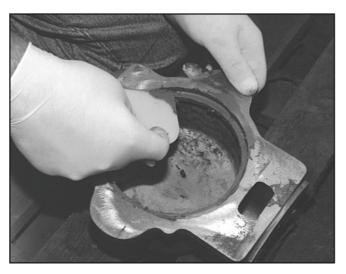
BRONZE PUTTY is a bronze filled epoxy putty designed especially for patching, filling and repairing castings, equipment and generally, components made from bronze or other similar alloys. It cures to a tough inert material that can be easily machined, drilled or tapped to any required tolerances.
