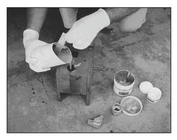
ALUMINIUM LIQUID is a pourable aluminium filled liquid epoxy that can be used in casting and moulding applications or in the repair of aluminium components and equipment. It cures to a tough inert material that is non rusting and can be easily machined, drilled or tapped to any required tolerances.
