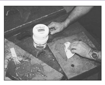
FAST STEEL PUTTY is an extremely fast curing steel putty designed to be a highly effective repair compound that enables emergency repairs to be carried out with minimal down time. It will even cure at very low temperatures to a tough inert material. It can be easily machined, drilled or tapped to the required tolerances after curing if necessary.
