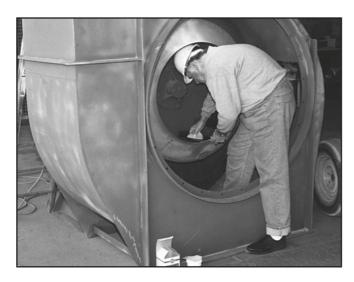
HIGH TEMP AR (Abrasion Resistant) PUTTY is a fine grade, trowellable, abrasion resistant epoxy for use on equipment prone to wear and corrosion whilst operating at extremely high temperatures. The special resin base which contains a blend of specially graded ceramic particles ensures outstanding chemical resistance with maximum protection in high wear applications.
