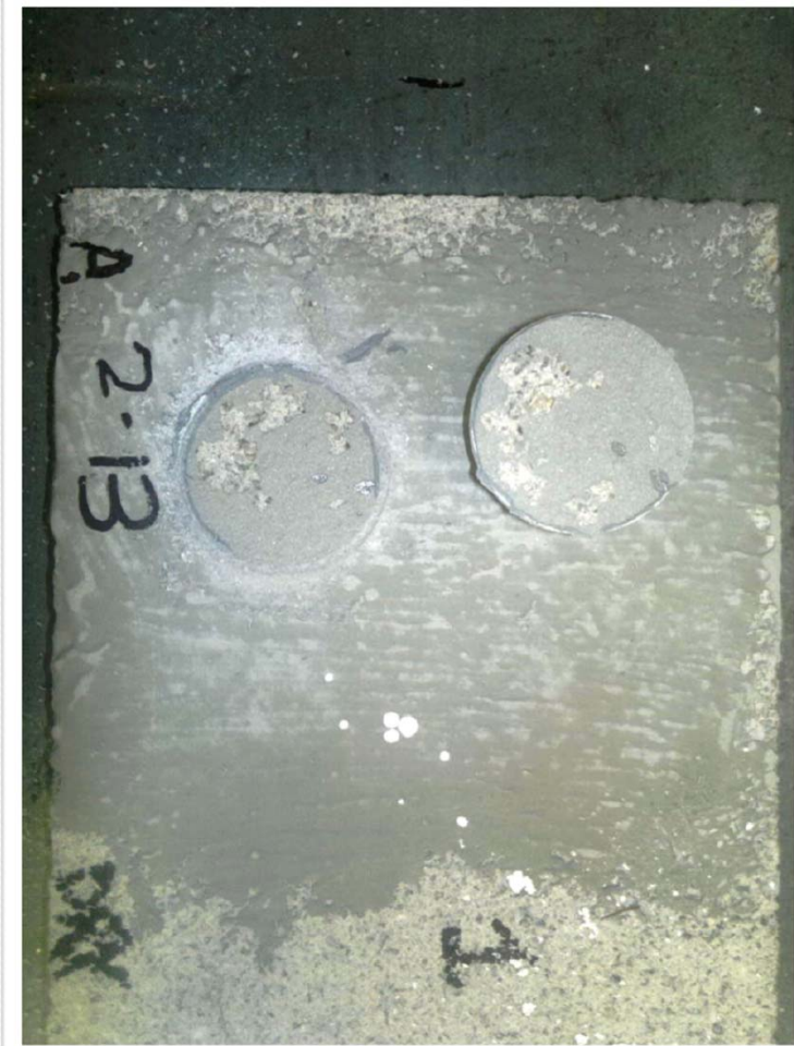
Polymer modified cement to dry concrete.
