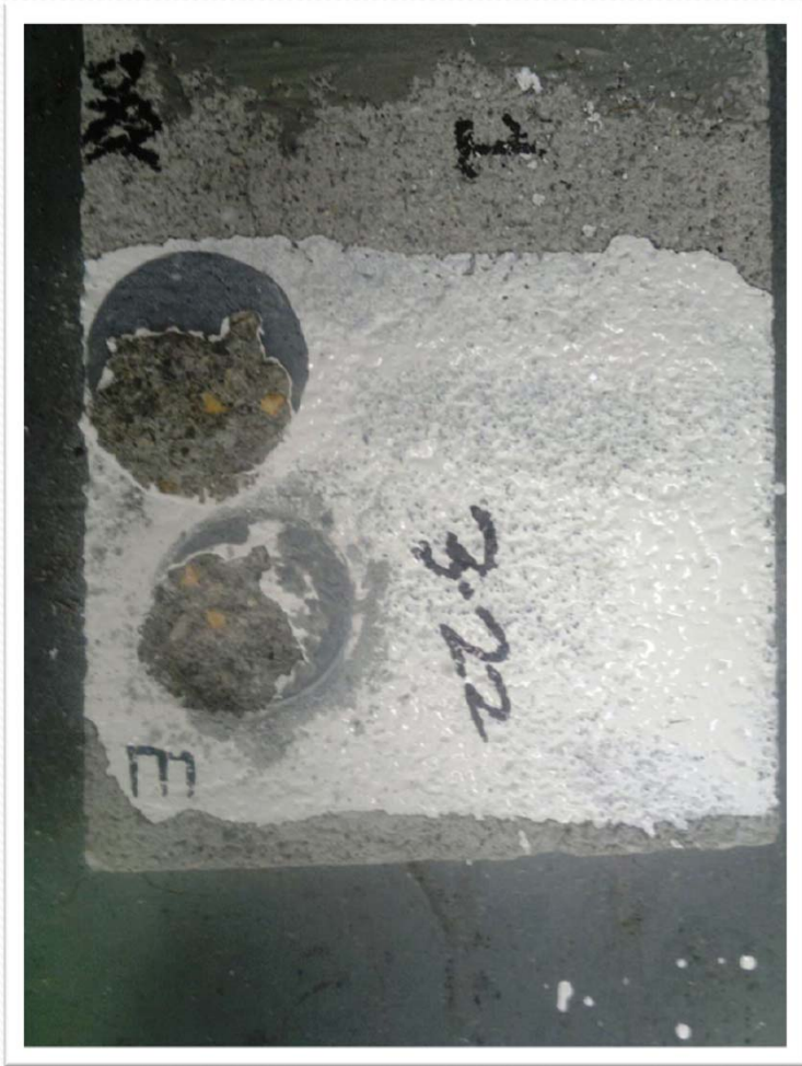
Solvent based standard epoxy to dry concrete.
