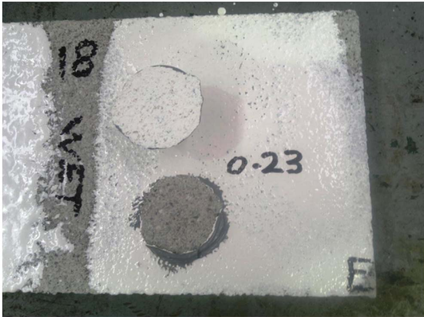
Solvent based standard epoxy to wet concrete
