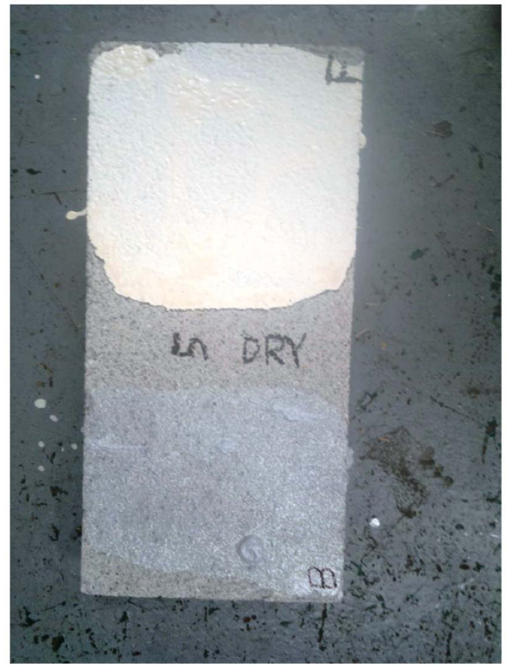
Top: Solvent containing epoxy novolac. Bottom: Water dispersed system.
